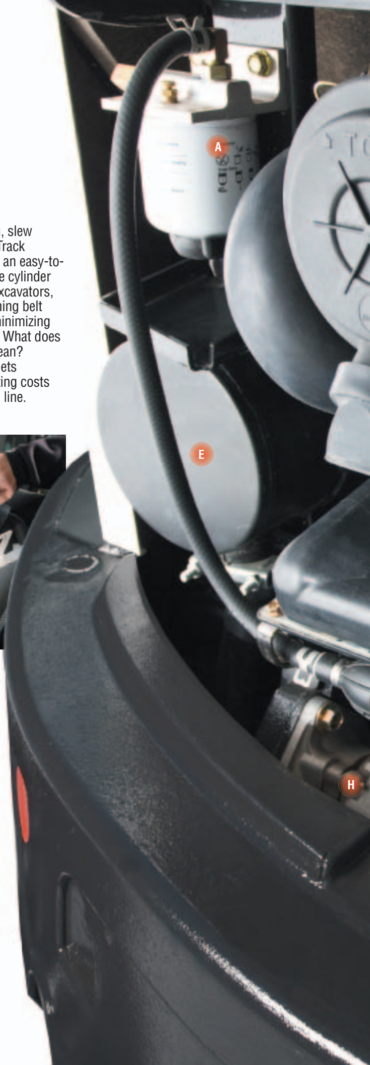
The cooling cores can be separated for quick, easy cleaning of the radiator.
