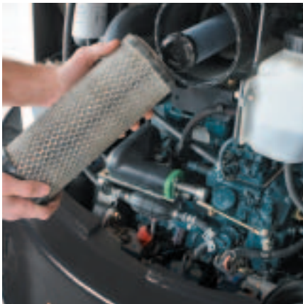
Time is money. Routine maintenance is an important factor in controlling operating costs. With Bobcat® excavators, filters, fluid, and daily maintenance checkpoints are right at your fingertips.
