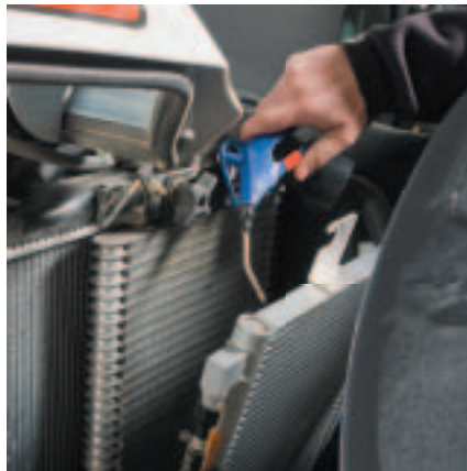
The cooling cores can be separated for quick, easy cleaning of the radiator.
